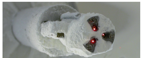
Fig. 2: 3-channel probe tip with patented pneumatic cleaning unit keeping the sensors clean of sticky maize starch.
