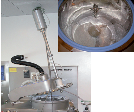
Fig. 4: Test arrangement at Roche's with Labasys®100 (left) and the inside of the high speed mixer (right).
